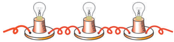
Fig. 12 - Bulbs connected in series
